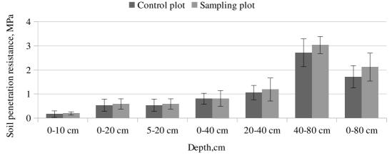
Fig. 2. Soil penetration resistance before compaction
