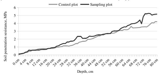
Fig. 3. Soil penetration resistance before compaction
