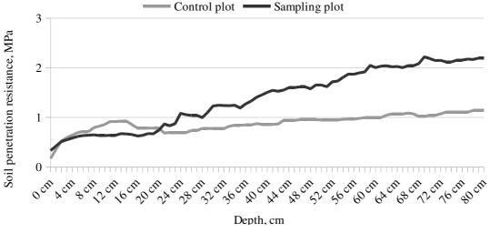
Fig. 4. Soil penetration resistance after compaction in sampling plot
